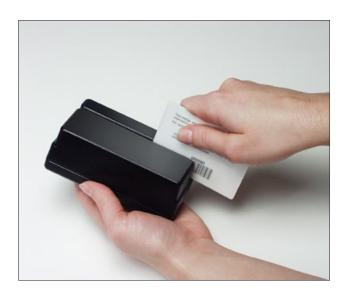
The Magbar DC is a dual-technology barcode/magnetic stripe data collection reader. It is available in fixed mount and portable versions. The portable version is especially convenient for collecting attendance at training classes. The fixed mount version can be wall mounted for time and attendance applications, and is available with POE.
