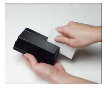
The Smart Mag DC is a data collection reader available in fixed mount and portable versions. The portable version is especially convenient for collecting attendance at training classes. The fixed mount version can be wall mounted for time and attendance applications, and is available with POE.
