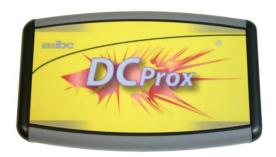
Easily collect user attendance at any function. The DCProx can hold thousands of scans with optional date and time stamping. Data can easily be uploaded to a PC. Powered from 2 AA batteries, USB, or AC adapter. Easy on/off switch.
