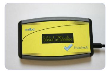
Easily identify and validate your proximity cards and fobs with Proxcheck. Proxcheck displays the card data in binary, hexadecimal and numeric formats. The Proxcheck reads cards up to 64 bits in size. Useful for field diagnostics and identifying card numbers for cards with worn-off printing.
