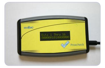
Easily identify and validate your Iclass cards and fobs with Proxcheck-IC. Proxcheck-IC displays the card data in binary, hexadecimal and numeric formats. The Proxcheck-IC reads cards up to 64 bits in size. Useful for field diagnostics and identifying card numbers for cards with worn-off printing.
