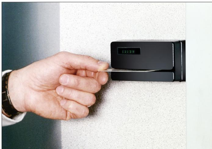
The Smart Slot STAx is a stand alone barcode reader with internal memory, timeclock, and audit trail. The reader contains an internal relay which is used for door control. Access is controlled by validation of badge numbers stored in the internal memory of the reader. Valid numbers can be downloaded into the reader from a PC or scanned into the reader by hand.
